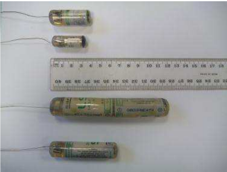
Figure 3. The size range of radio transmitters used in the study.
