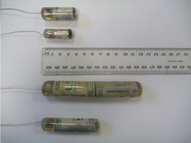
Figure 3. The size range of radio transmitters used in the study.
